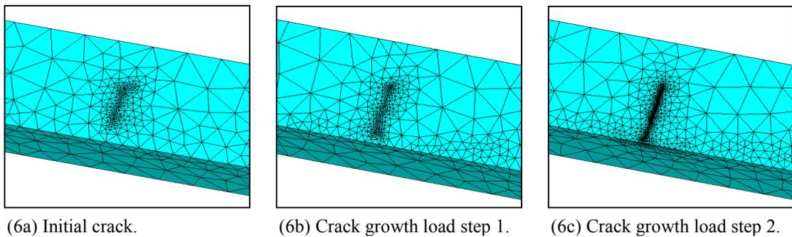
**Figure 6 Surface crack propagation.**
