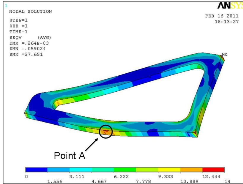
**Figure 4 Stress distribution of the unnotched bracket (Von Mises).**
