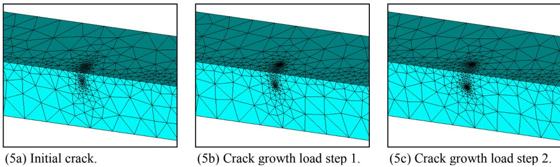
**Figure 5 Corner crack propagation.**
