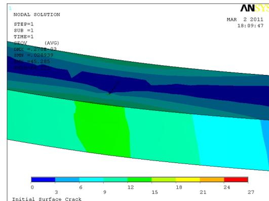
(7b) Surface crack stress field.
