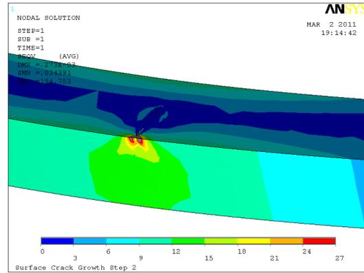
(8b) Surface crack stress field.
