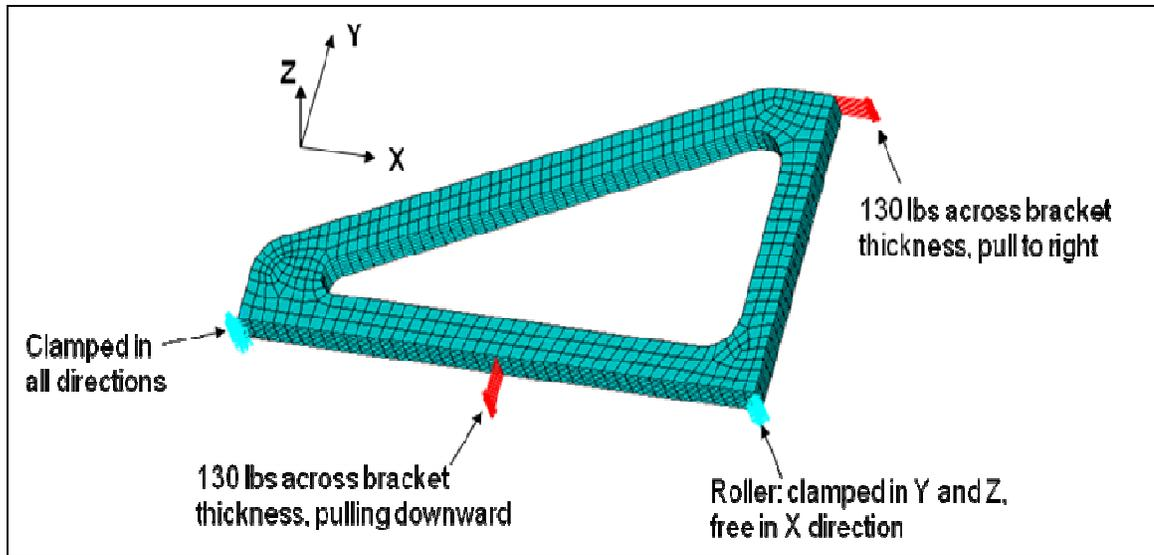
**Figure 3 The boundary conditions of the unnotched bracket.**
