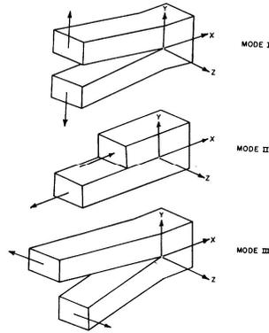
**Figure 1 The three basic modes of crack surface displacements [5].**
