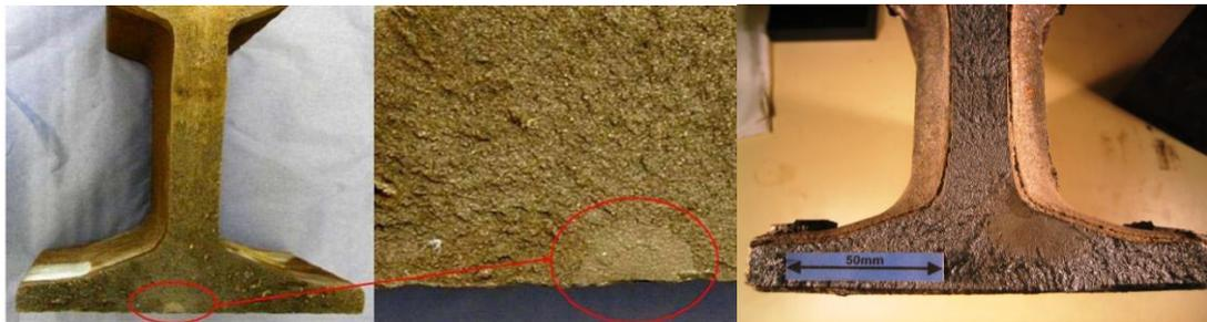
Figure 2. Flaws on fatigued samples, semicircular crack at rail base (left), elliptical crack at bottom web corner (right)
