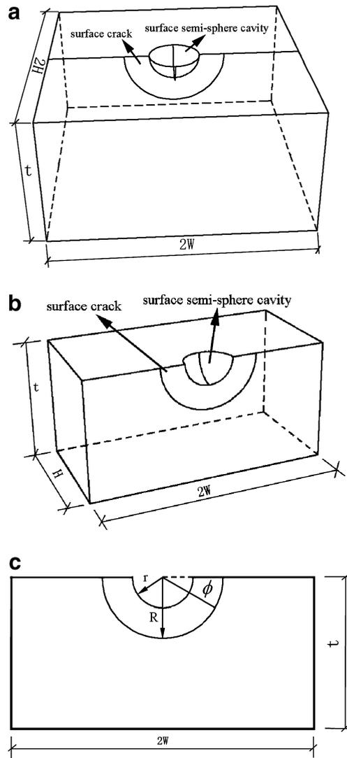
Fig. 1. Schematic of cracks emanating from a surface semi-spherical cavity in infinite elastic body: (a) total view, (b) local view (a half of Fig. (a)) and (c) the symmetry plane in which the crack surface occurs.
